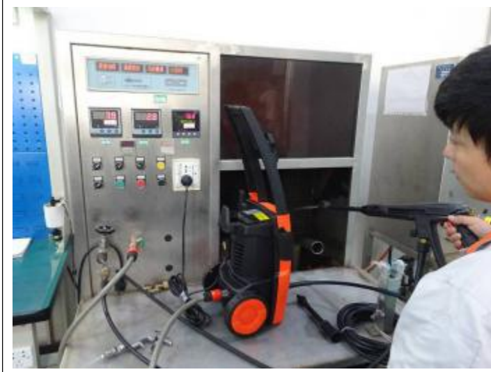
138. Max water Flow Rate Test
